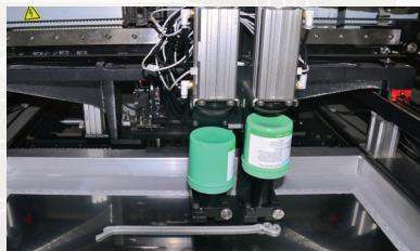
Dispense for standard cartridges or choose the new patent-pending jar dispenser. Paste is released in precise, measured amounts across the stencil in a clean, uniform bead. Deposition volumes, frequency and placement are user programmable.
