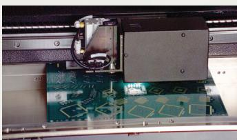
MPM's patented printer-based Vision and Inspection system is a cost-effective way to verify print and paste deposit results. It is flexible enough to handle the complete range of today's most challenging components. This system measures the amount of paste covering the target pad and compares it with the required coverage. 2D inspection is integrated directly into the stencil printer to provide an immediate source of data.
