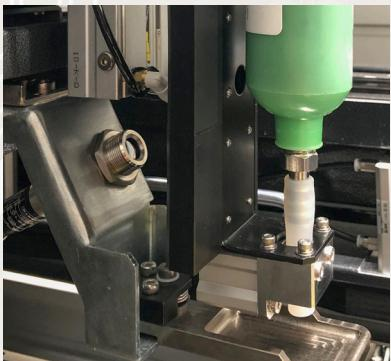
Temperature monitoring ensures proper paste viscosity to avoid bridging and voiding. MPM patent-pending paste temperature monitor allows paste to be measured in the cartridge or on the stencil.
