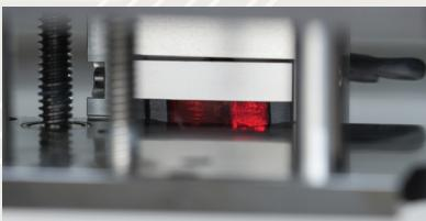
The Paste Height Monitor is designed to prevent defects caused by inadequate volumes of paste on the stencil. It combines advanced
