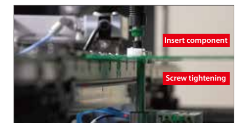
One unit can insert component and screw tightening
